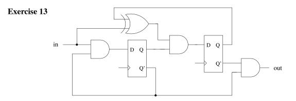
Draw an I/O-automaton modelling the digital circuit shown above. Use  $\Sigma := \Theta := \{0, 1\}$  as inputand output-alphabet.
