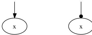
Figure 3.1: Graphical representation of x (left) and \neg x (right) by an AIG
