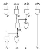
$$\begin{array}{lll} s_3 = g_1 \wedge g_4 & -s_3 + g_1 g_4, \\ s_2 = g_1 \oplus g_4 & -s_2 + g_1 + g_4 - 2g_1 g_4, \\ g_4 = g_2 \wedge g_3 & -g_4 + g_2 g_3, \\ s_1 = g_2 \oplus g_3 & -s_1 + g_2 + g_3 - 2g_2 g_3, \\ g_1 = a_1 \wedge b_1 & -g_1 + a_1 b_1, \\ g_2 = a_0 \wedge b_1 & -g_2 + a_0 b_1, \\ g_3 = a_1 \wedge b_0 & -g_3 + a_1 b_0, \\ s_0 = a_0 \wedge b_0 & -s_0 + a_0 b_0 \end{array}$$
